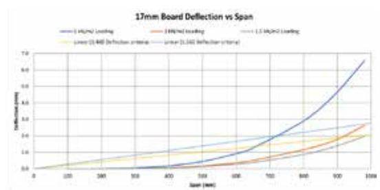
The deflection chart indicates the amount a decking board will deflect, between joints, when subject to a distributed load. Point loads will cause greater localized deflection of the boards.
