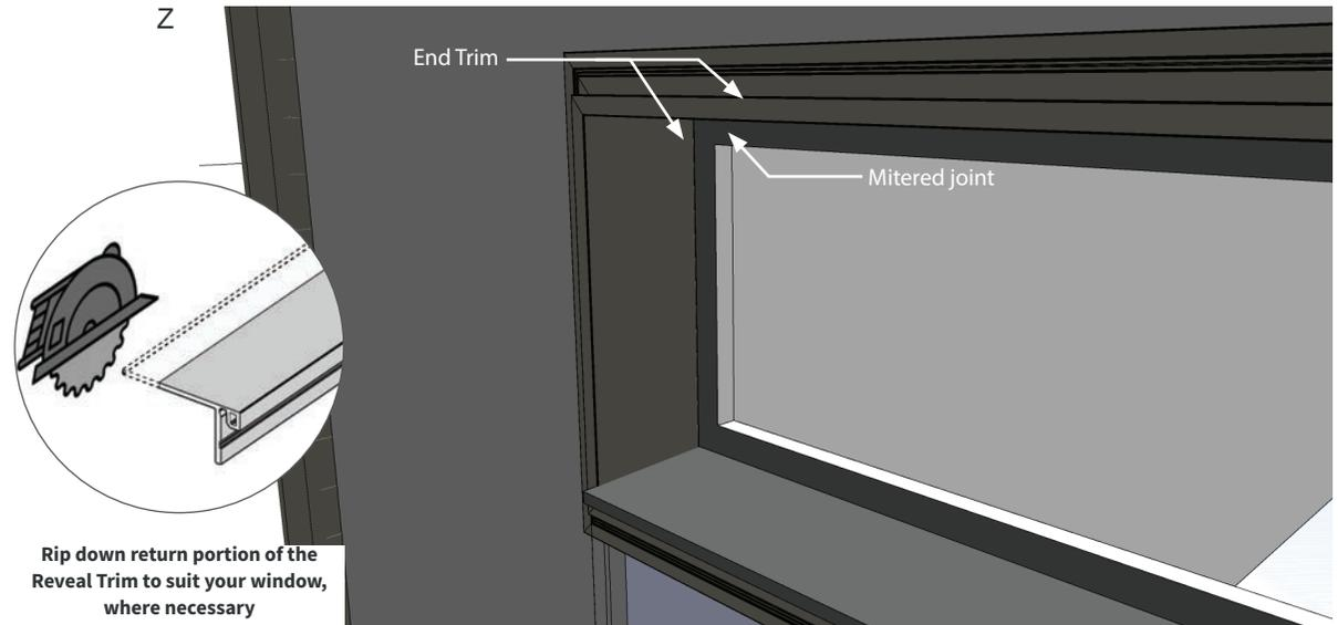
A1 Cladding can then be laid around the window and the joints around the frame sealed with colour matching mastic to achieve a neat finish.
