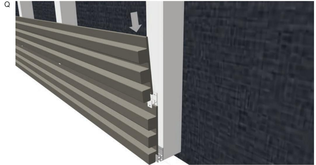
R Where boards meet end to end, ensure the appropriate expansion gap is left between boards. Refer to the table on page 54 for distances.
