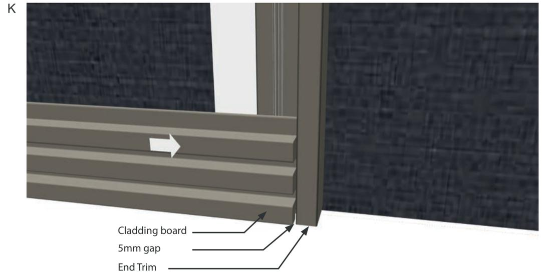
L Boards which abut a corner trim should be positioned 5-7mm away from the corner trim batten face – as shown in the diagram. This is to allow the board to sit flush against the trims back face, and not ride up on the trims profile.
