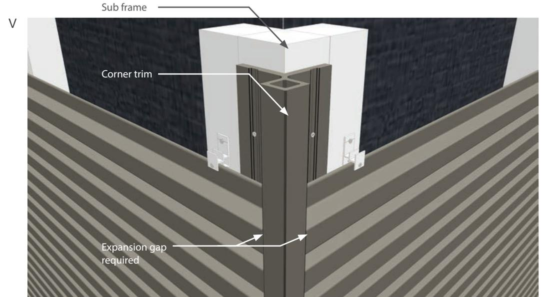
W Where cladding panels run into a wall or post, an end trim is not always required. Just ensure an expansion gap is left between the end of the board and the face of the wall. Refer to page 54 for distances.
